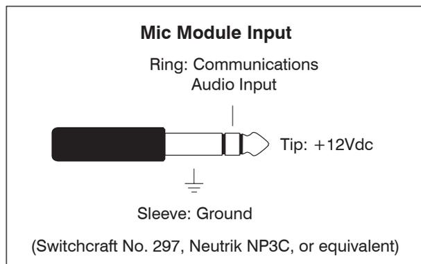
ground on sleeve. The audio input requires a nominal -10dBu signal (-10dBu, not -10dBV!). The +12Vdc on the tip is from the same source that powers the Model 51, and is provided to power an external preamp. If you feel the urge to use this power source, be aware that it only provides 110 milliamps of current of which the Model 51 needs about 100mA. So go ahead and use all the current you need, as long as it doesn't exceed 10mA!
