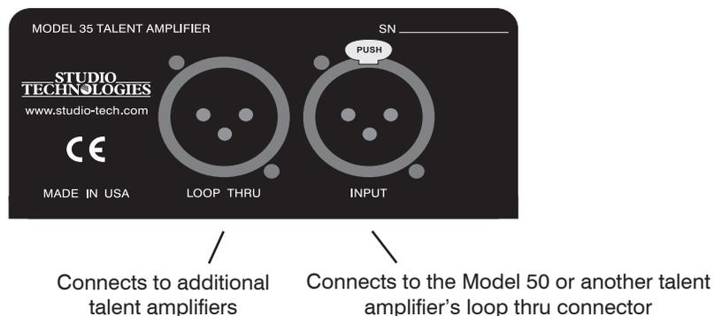
allows a musician's microphone or line-level signal to be "looped" through the Model 38, boosted by its preamp, and then combined with the stereo cue mix supplied by the Model 50. This provides each Model 38 with an individual headphone mix, solving the classic problem of wanting "more me" in the phones! Like the Model 35, the Model 38 is linked with a Model 50 Central Controller by a single cable.
