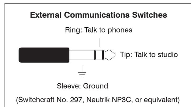
Switchcraft No. 297, Neutrik NP3C, or equivalent will work correctly. Use a momentary, single-pole, single-throw switch for each remote function. The respective function is activated when the tip or ring get shorted to the sleeve.
