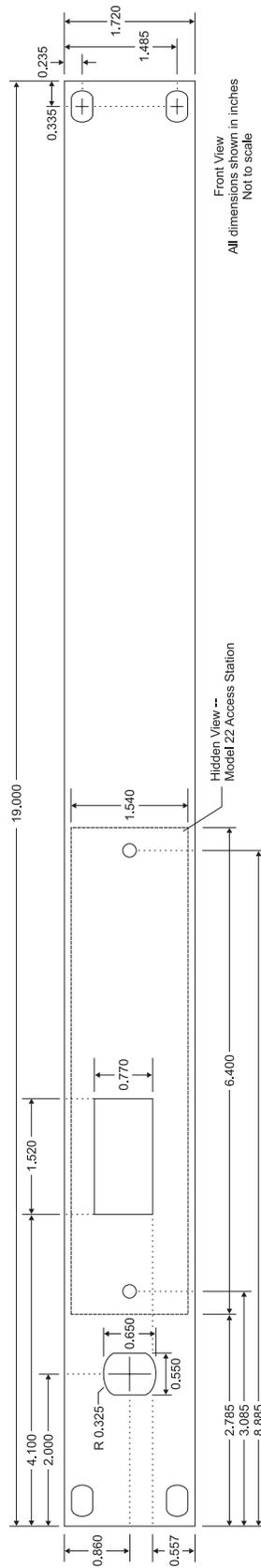
Figure 4. IFB Plus Series Model 22 Access Station Overall Dimensions
