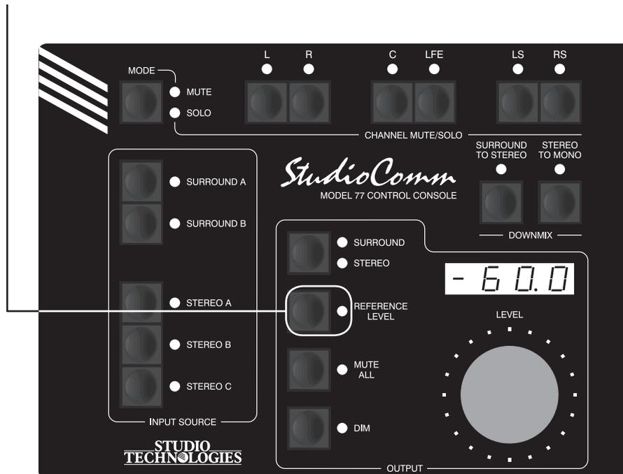
**Default:** Reference level set for -60.0 dB post-fader monitor output level.
