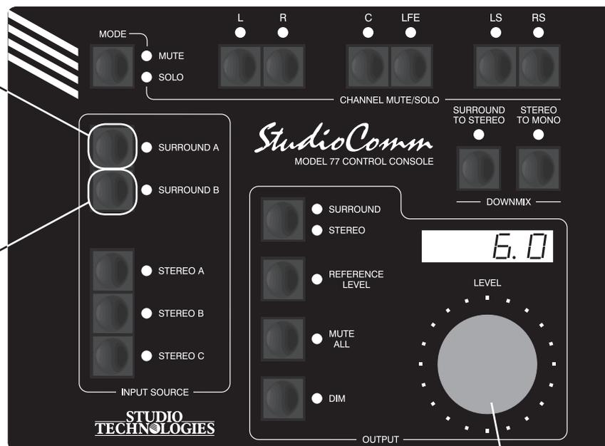
When the Surround A button is pressed, use the level control to adjust the **channel pop solo up offset level**. The range is 0.0 to 12.0 in 0.5-dB steps.
