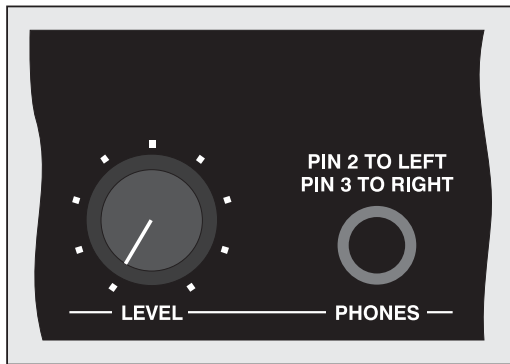
Figure 8. Detail of front panel showing headphone section
