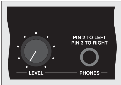
Figure 8. Detail of front panel showing headphone section
