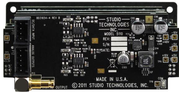
Model 5110 Mic/Line Input Module Back View
