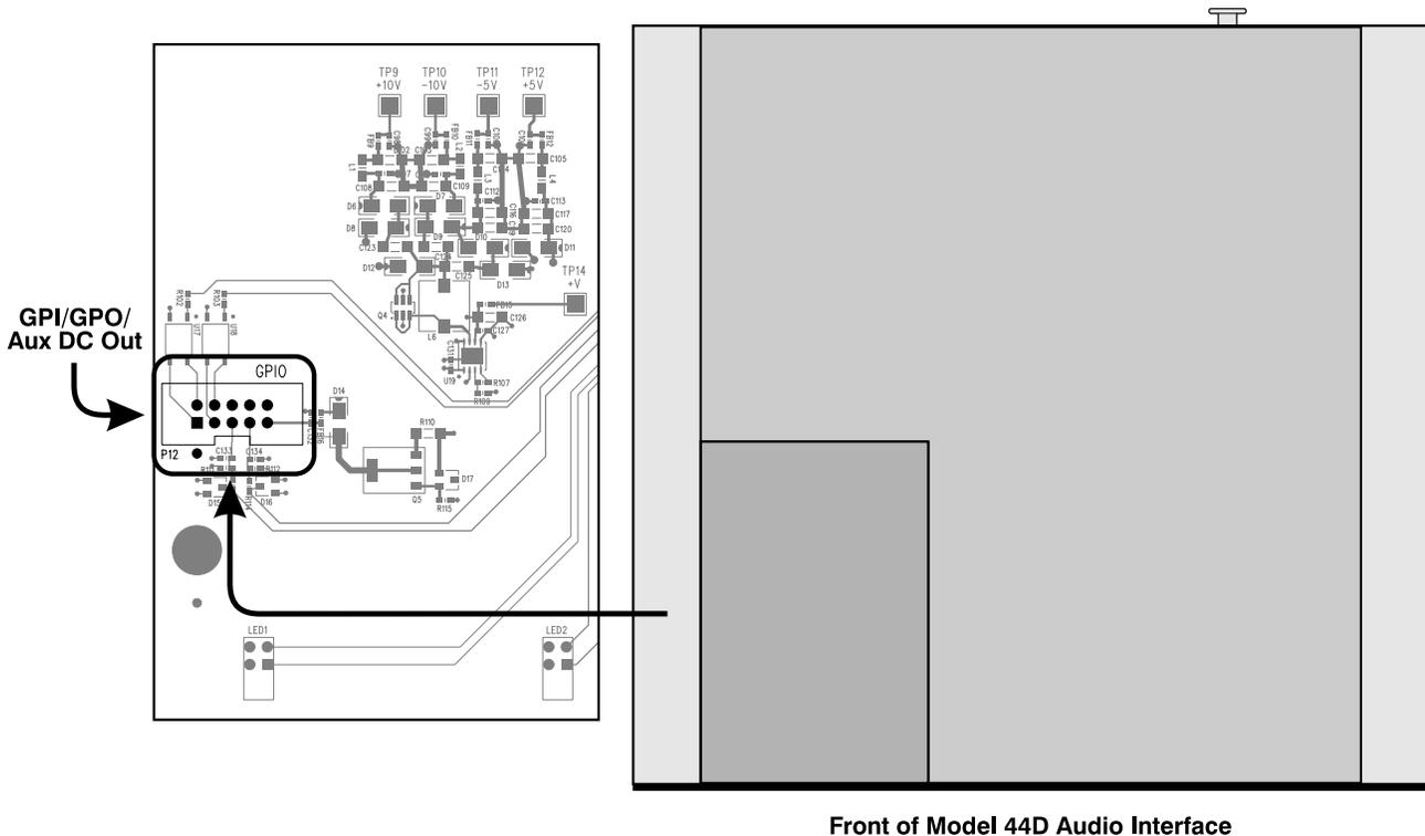
**Figure 9. Model 44D GPI/GPO/Aux DC Out 10-pin header location (applies to M44D-00151-00250)**
