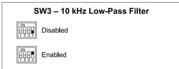
**Figure 6. 10 kHz low-pass filter configuration switch**
