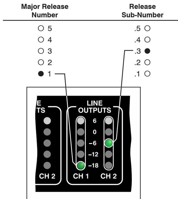
**Figure 7. Detail of front panel showing the status LEDs that display the application firmware version. In this example, the application firmware version is 1.3.**
