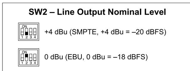
**Figure 5. Analog outputs nominal level configuration switch**
