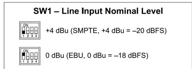
**Figure 4. Analog inputs nominal level configuration switch**
