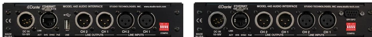
**Figure 8. Back view of “original” Model 44D unit with serial numbers 00151-00250 (left) and “updated” Model 44D unit with serial numbers 01151-later (right)**
